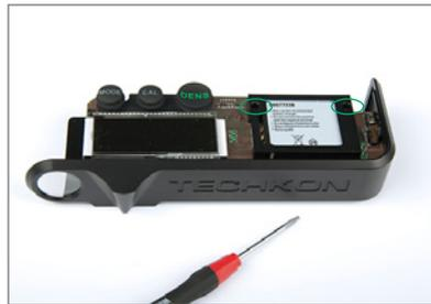
1. Unscrew the three TORX™ screws on the device bottom and remove the upper device case.
